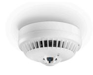
Intelligent optical and thermal multi sensor detector for Loop 3000 with two optical and two thermal sensors and a bidirectional isolator for earliest fire detection and indication in all environments with difficult ambient conditions, according to EN 54-5/-7 /-17, prEN 54-29 and CEA 4021
